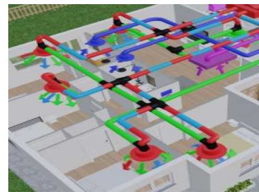
In Ceiling system layout
